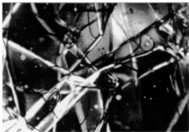
Figure 10. Light microscopy photo of dry C25DMAm SIPN film (200 \times ). Figure reduced to 75% for publication.
